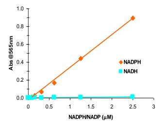
Fig 1. NADPH and NADH were serially diluted in assay buffer containing Enzyme Cycling Mix and Detection Reagent, followed by addition of stop solution. Absorbance was recorded at 565 nm. (Ultra Microplate Reader EL808, Bio-Tek Instruments, Inc).
