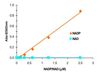
Fig 2. NADP and NAD were serially diluted in assay buffer containing Enzyme Cycling Mix and Detection Reagent, followed by addition of stop solution. Absorbance was recorded at 565 nm. (Ultra Microplate Reader EL808, Bio-Tek Instruments, Inc).
